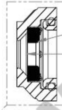
Proper DLFC orientation directs water flow towards the washer face with rounded edge
